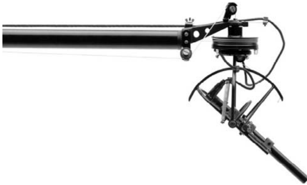
FIGURE 4.2 The business end of a Fisher boom, showing the mechanism that rotates and tilts the microphone under the control of the operator at the other end of the boom. Photo courtesy J. L. Fisher, Inc.
