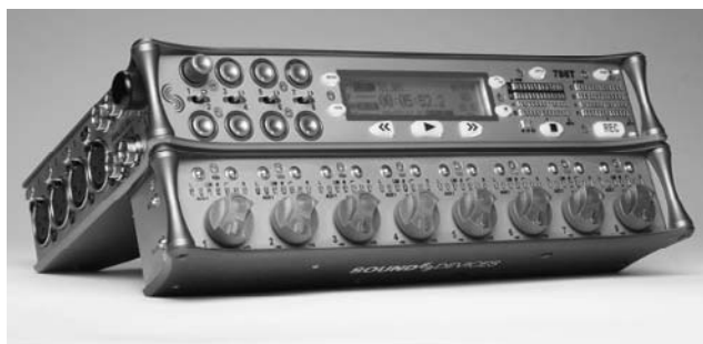
FIGURE 7.3 A Sound Devices 788T with accessory controller CL-8. Photo courtesy Sound Devices LLC.
